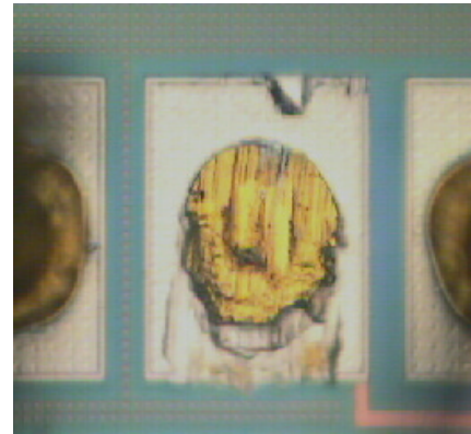
Ball Shear Strength/Area = 5.5gf/mil 2
