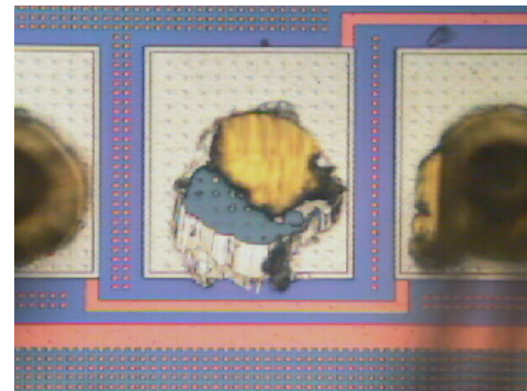
No Pad Lift
