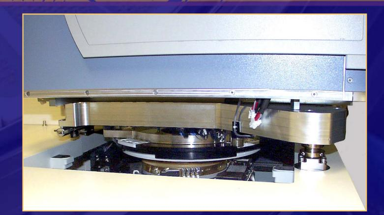
The Z-reference for the probe card is built into the spring contact assembly
