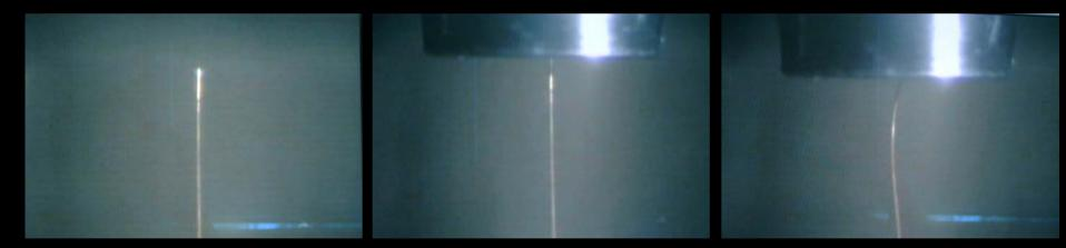
Probe pin deforms with buckling modeScrub motion of the pin point is small.
