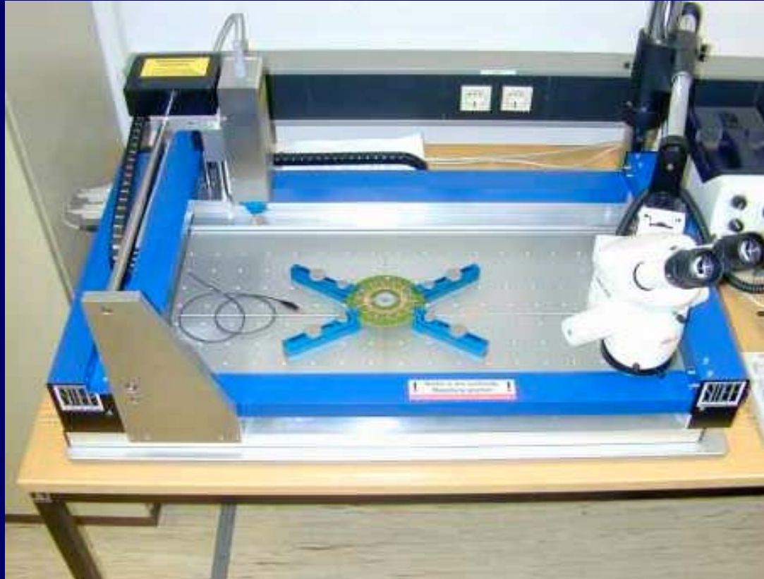
T.I.P.S. "Probe Refresher" machine
