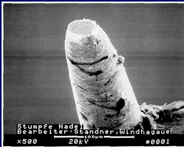
flattened probe tip
