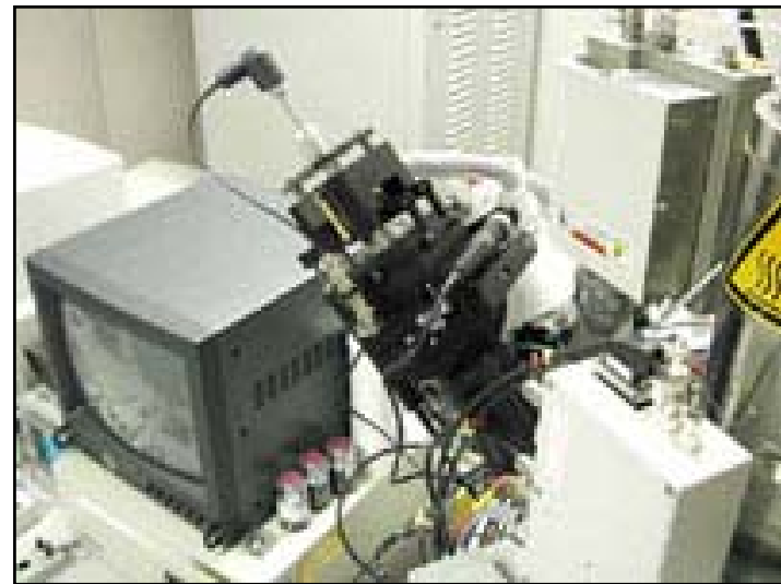
Omniprober mounted on FEI DB235 FIB
