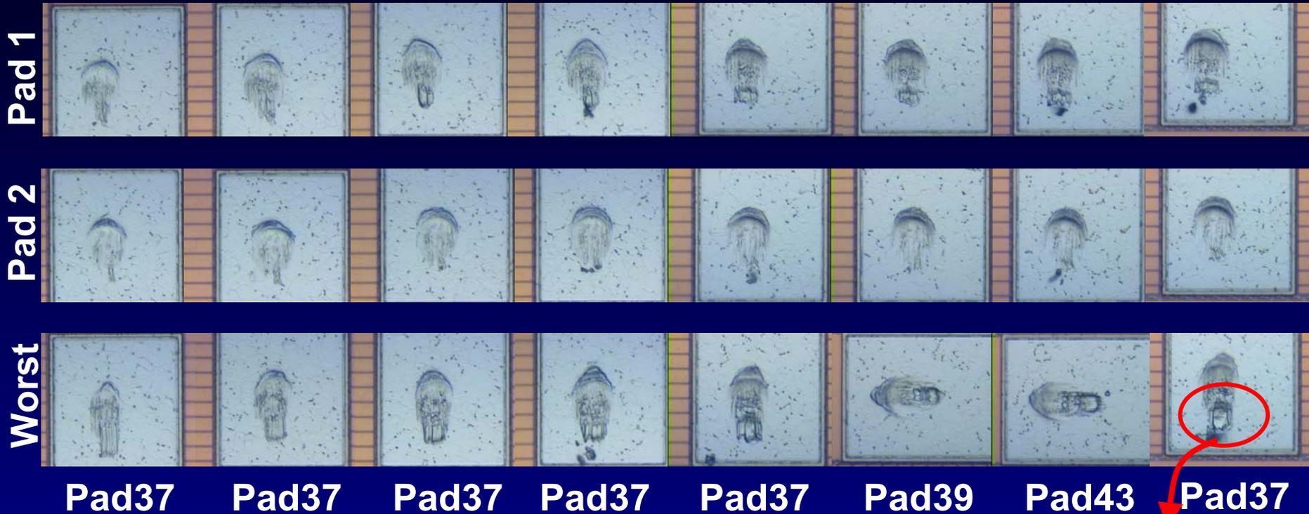
**Vendor A crack threshold moved beyond 3x TD, now at 7x TD.
