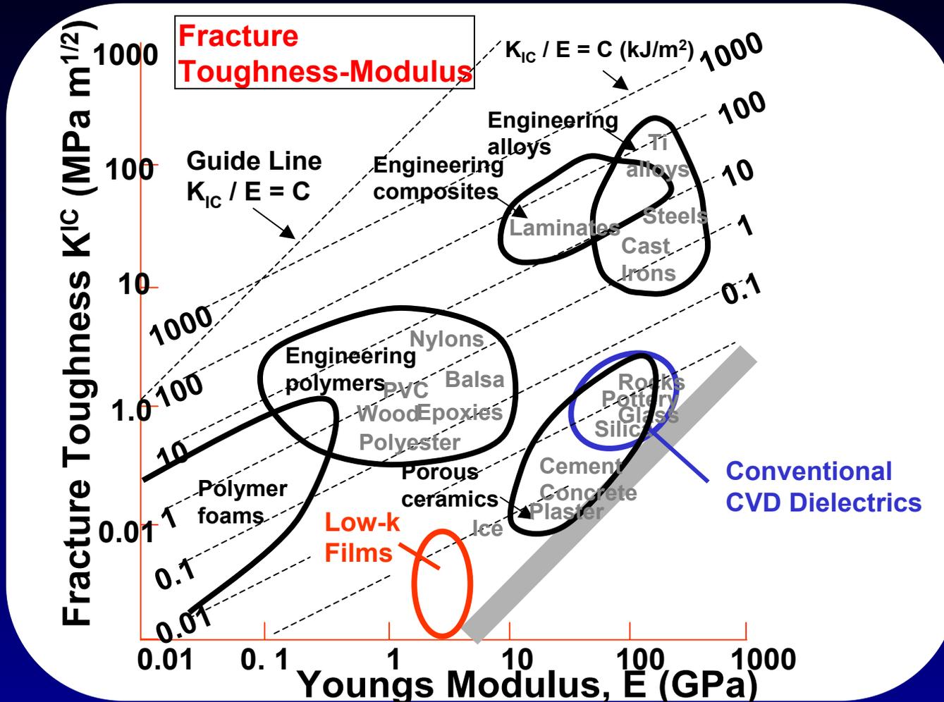
Low-k dielectrics are in a class of their own concerning combined modulus and fracture toughness properties.
