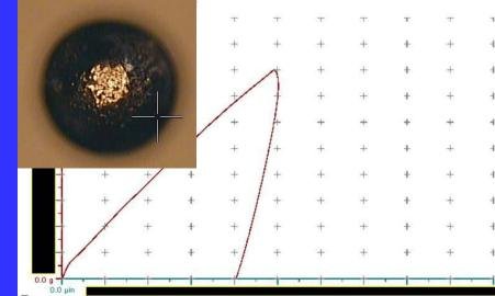
Impact of Pb-free conversion on the force required to successfully probe the FCP or an equivalent CSP. Also note the slope of the line changes on load and unload cycles demonstrating divergence in mechanical properties.
