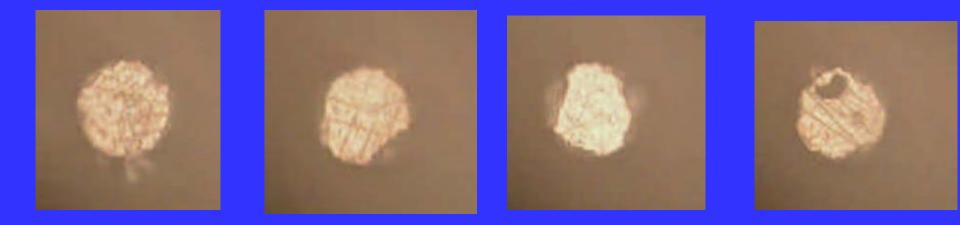
Cleaning friction profiles can be the death of a probe card. The tips show that various cleaning solutions, after only a few <u>cleans, have minor to major impact on</u> <u>needles</u>.
