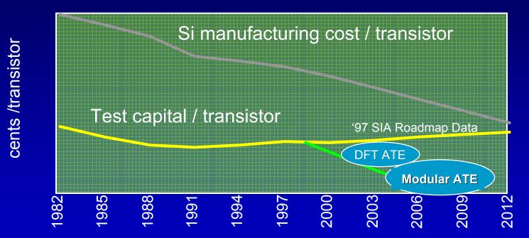
DFT & Structural Test reduce equipment cost & complexity
