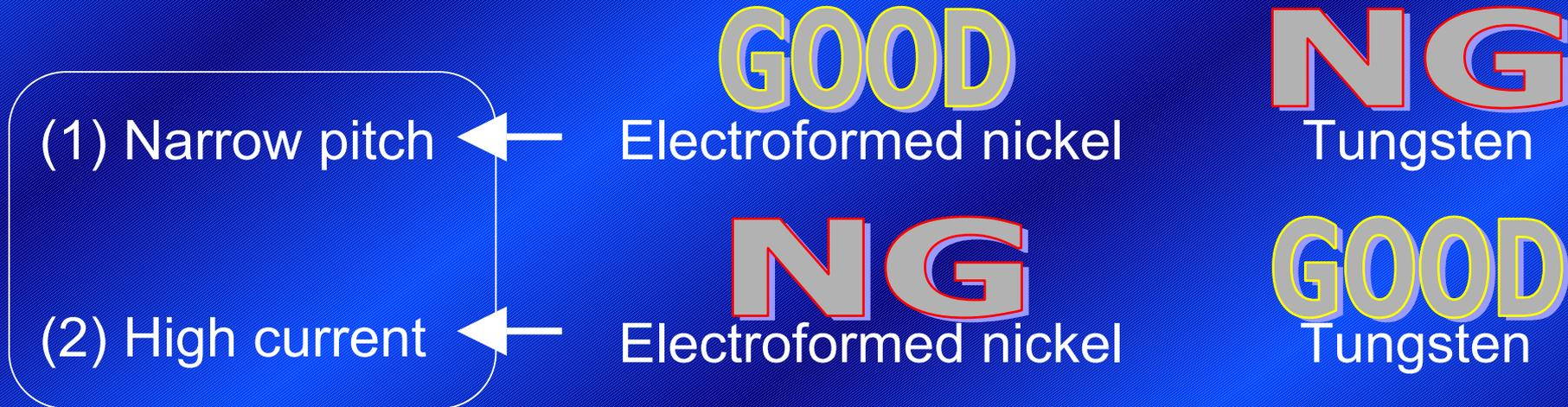
New material for advanced probe is required !
