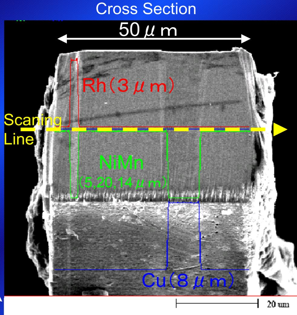
Overall resistance is calculated as 83% of Ni-Mn probe !
