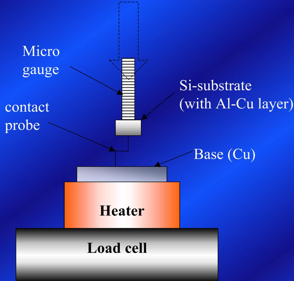
Schematic view of measuring system
