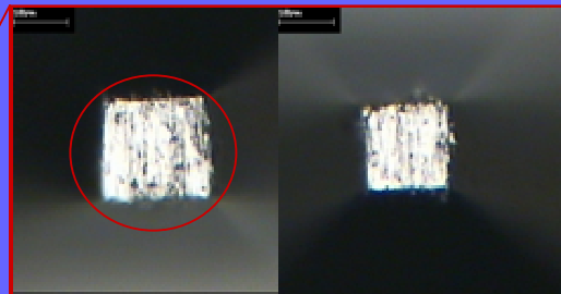
tip size max. 19mm end of live 22mm
