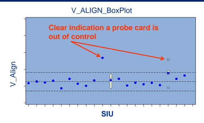
⇒Process control ensures both <u>tool</u> and <u>probe card</u> <u>fleet</u> are in control
