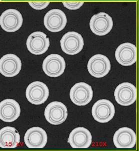
Wire Bond process control allows for consistent Stud Bump diameters which provides the opportunity for tight pitches
