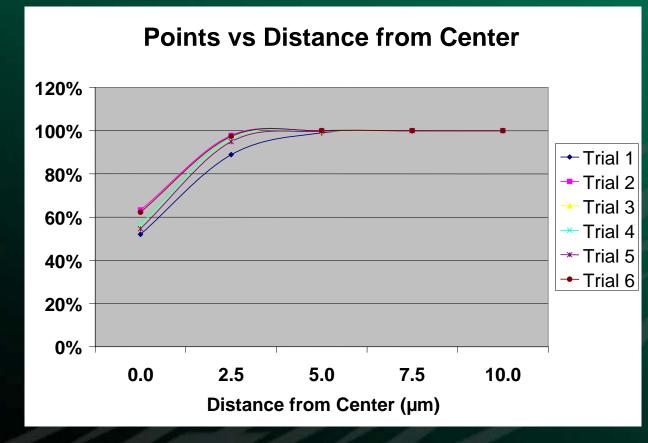
Pad Find Feature of the Wire Bonder is Accurate to 7.5 µm
