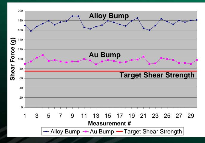
Stud Bump adhesion exceeds the target shear needed for lifetime
