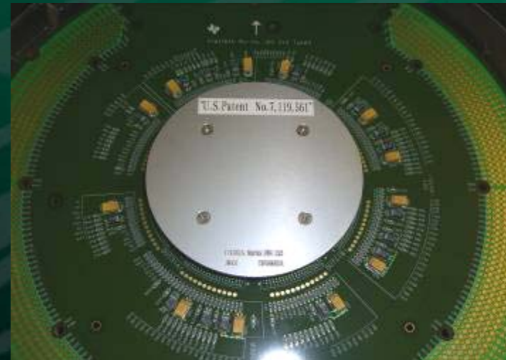
Probe card w/ Site Trace Length and Component Layout Matching
