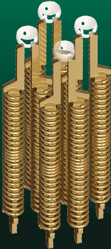
Probe pairs on 0.65 mm BGA
