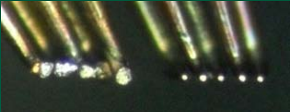
probe tip contamination
