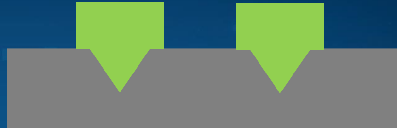
Fill with metal and build metal pillar
