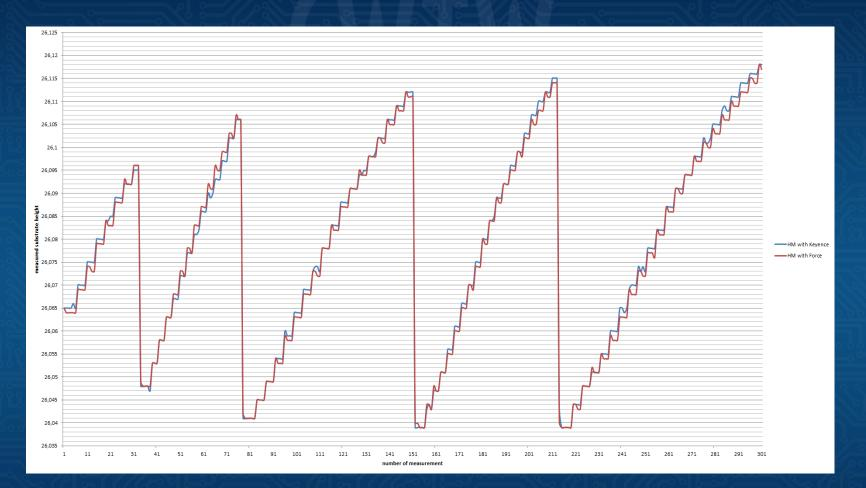
**Comparison Laser Measurement vs Force Measurement**
