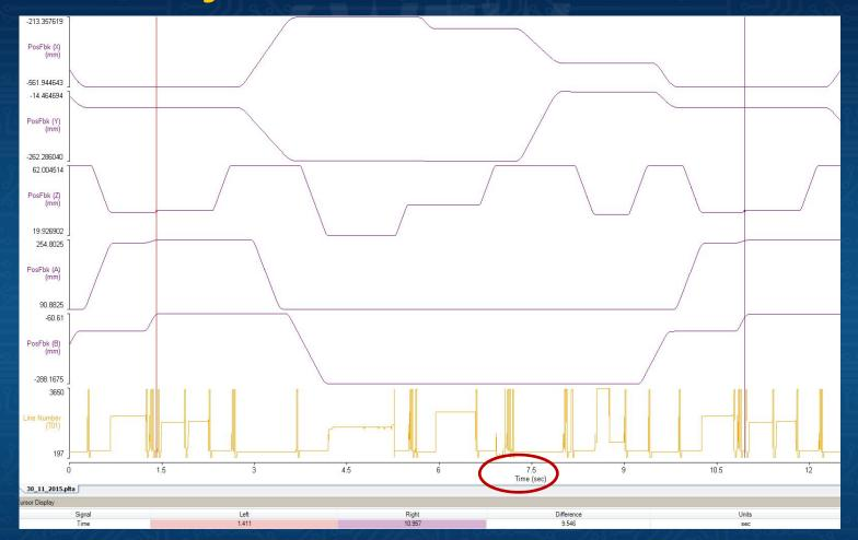
Complete process cycle time incl. Laser: 9,5sec
