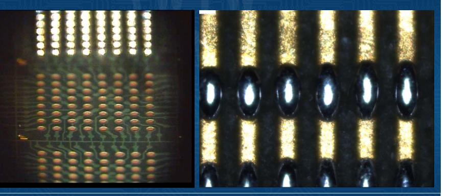
Solder depots placed on probe card substrate pads
