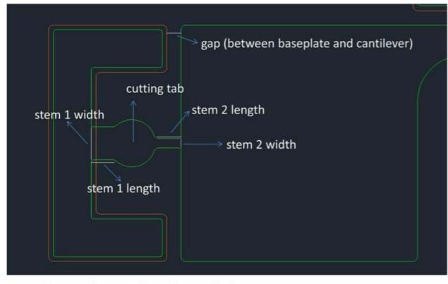
stem 1 – stem between baseplate and tab stem 2 – stem between tab and cantilever
