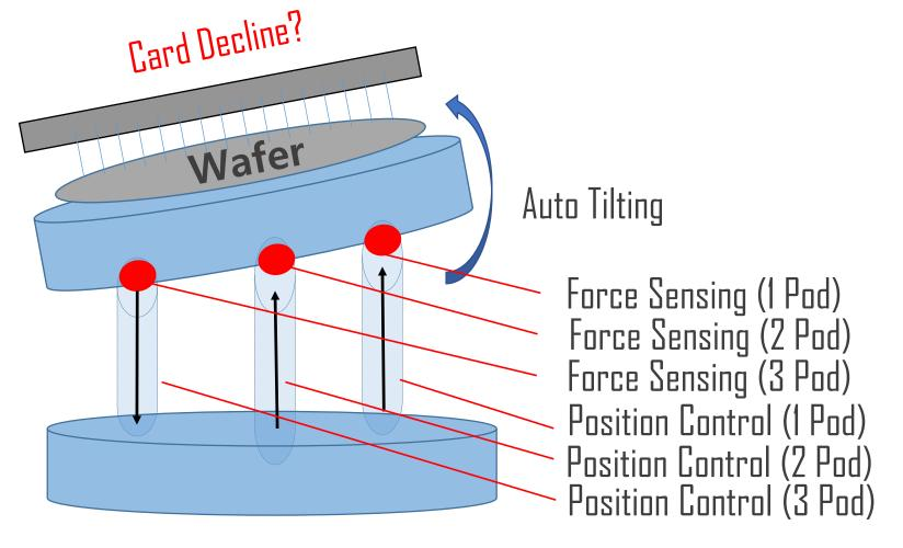
0 ~ 0.45 sec Block : First Contact at 1 Pod Position, 1 & 2 & 3 Pod Continue to Up ~ 0.7 sec Block : Second Contact at 2 Pod Position, 1 Pod Stop to Up, 2 & 3 Pod Continue to Up
