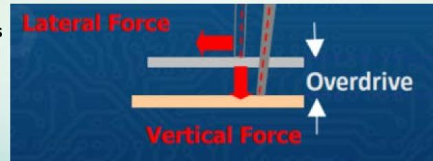
Heavy Vertical Force can crack the Inter-Layer-Dielectric (ILD)
