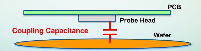
Take Away: eMantis probes lower coupling to wafer, which yields a truer data signature
