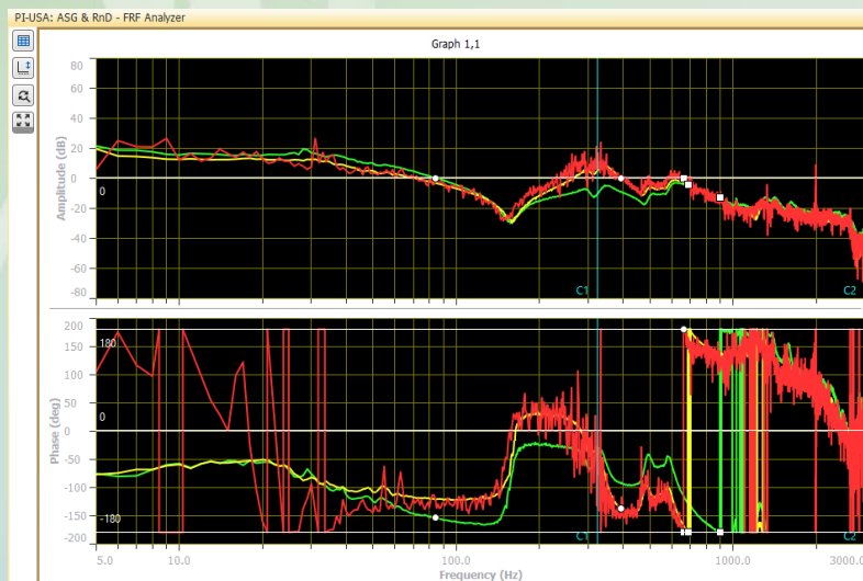
Figure 17. Transfer Function Characterization No Notch (Red) Notch Filter Applied (Yellow) Notch + Gains Optimized (Green)
