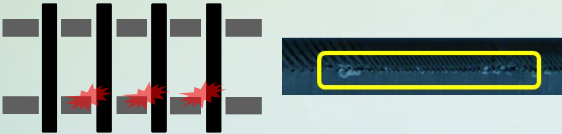
Ceramic crack due to high stress
