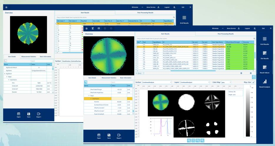
checking head flatness, tilt to tip plane, PCB & stiffener plane
