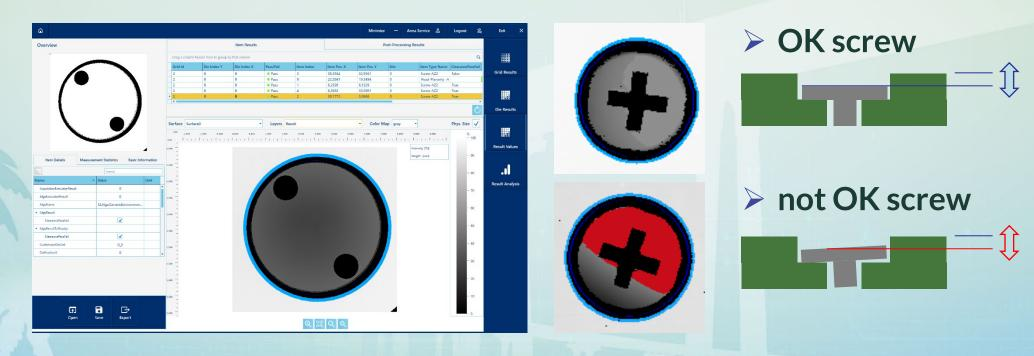
checking tip length, position, diameter, planarity
