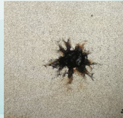
Fig. 4: "hot spot" damage on chip pad metal
