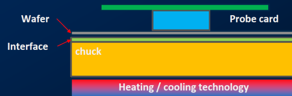
Schematic of a typical wafer prober, not drawn to scale
