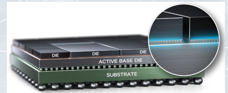
Illustration of a stacked die on a substrate
