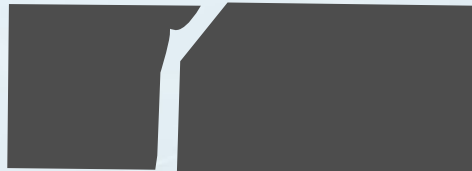
Complete Open of metal line Functional Fail
