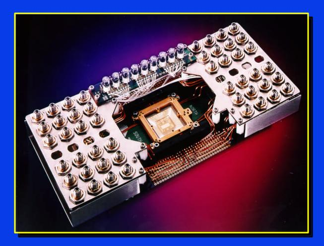
30 RF lines ~ 5 GHz • 200 AC lines ~ 500 MHz • 400 I/O solder ball arrays
