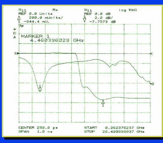
Time and Frequency response of standard bypass caps and low impedance power lines
