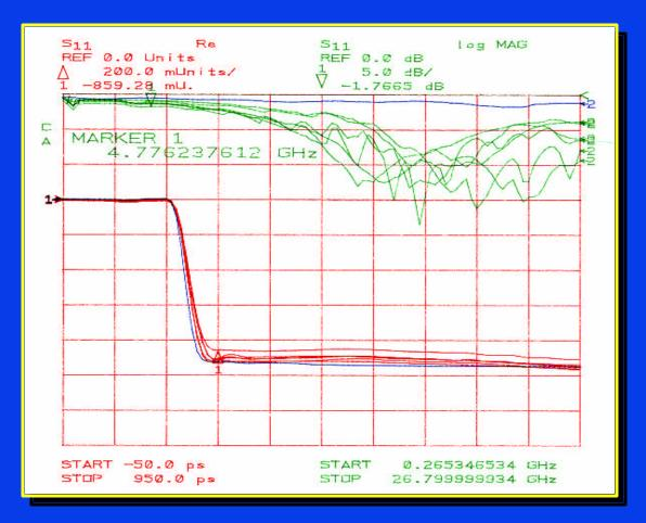
Time and frequency response of two stage bypass structure
