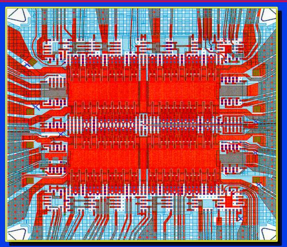
Interlaced power and ground planes •2 GHz atspeed test Minimal IR drop on supplies
