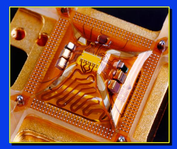
PCS Power amplifier for **CDMA** Impedance transformation from 2.5 to 50 ohms at 1900 MHz
