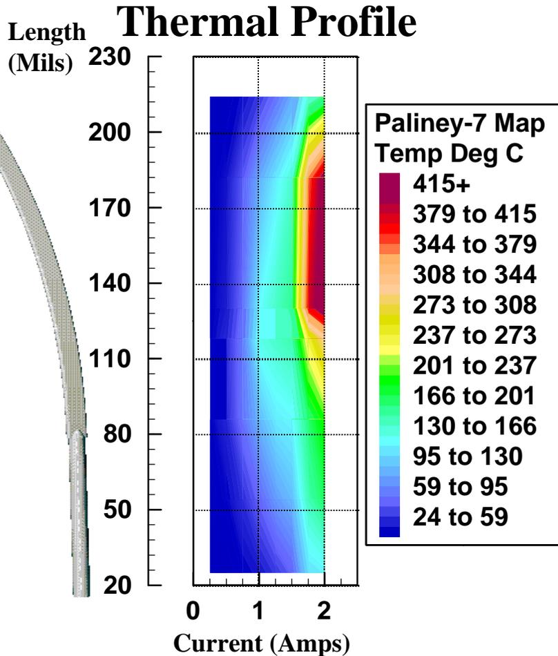
Figure 4 - Distributed Temp versus Current.
