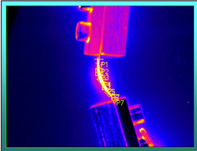
As the current is increased through the constriction, or probe ribbon, it will soon follow the  $I^2R$  heating until the formed region softens relieving the energy.
