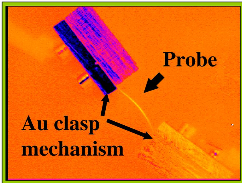
Figure 2 - Mounted Buckling Beam Probe.
