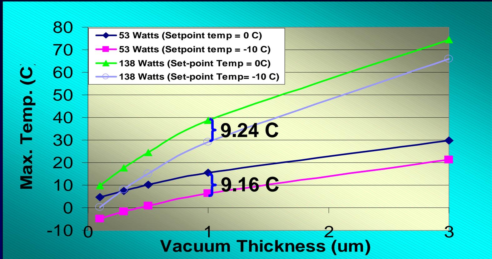
Changing the vacuum thickness from 0.1um to 3um and then, decreasing the set-point temperature of the chuck top from 0 C to -10 C decreases the Tj rise by ~ 9 C.
