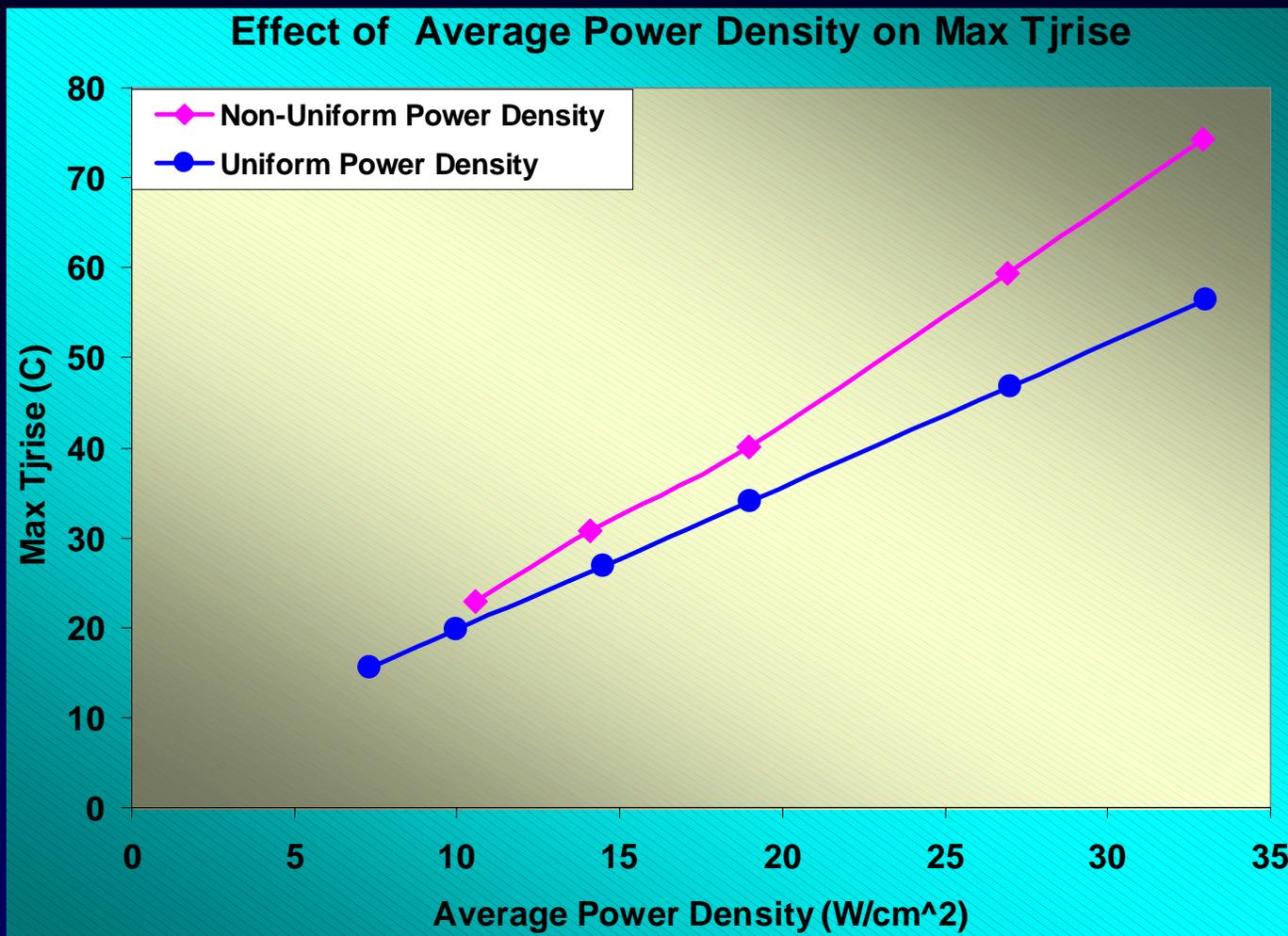
**At the same average power density, max Tjrise for a non-uniform power density is higher than the uniform power density.**
