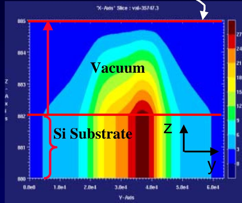
Sharp temp gradient between Si substrate bottom and top of the Chuck
