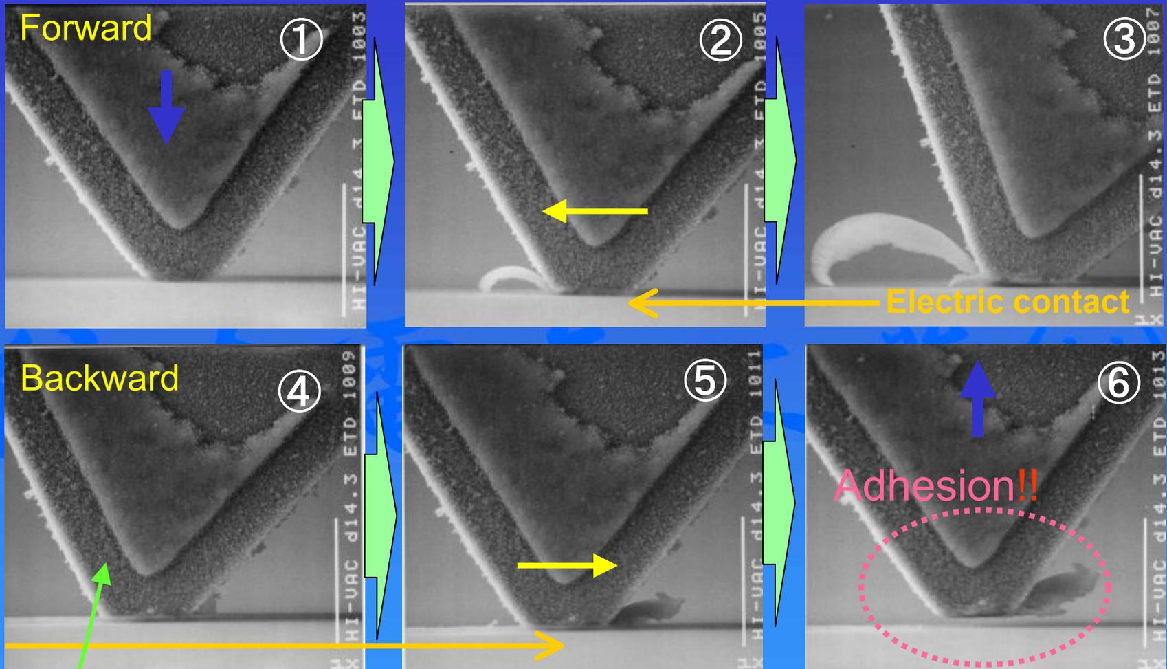
Probe Tip : Pillar-shaped structure imitated truncated pyramid tip
