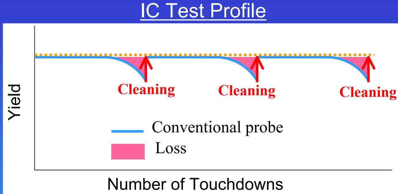
Adhesion and accumulation of debris at the probe tip
