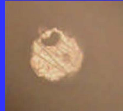
Cleaning friction profiles can be the death of a probe card. The tips show that various cleaning solutions, after only a few cleans, have minor to major impact on needles.
