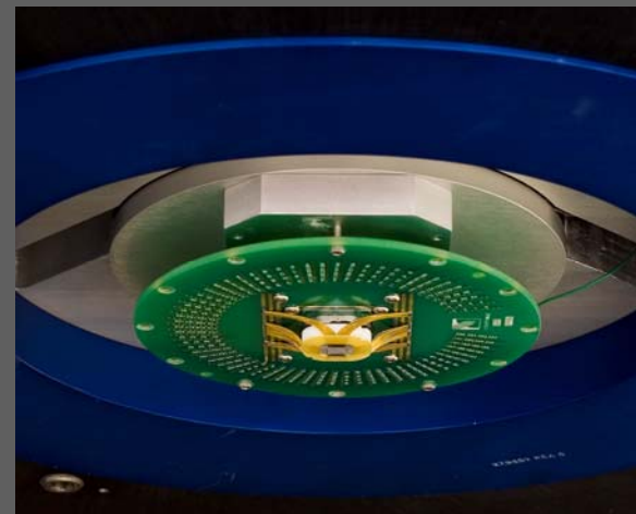
Probecard mounted on force sensor
