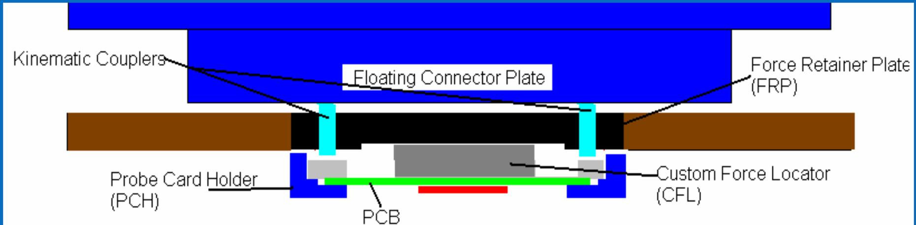
**Fig.1- Schematic of the interface of Test Head, FRP and CFL**
