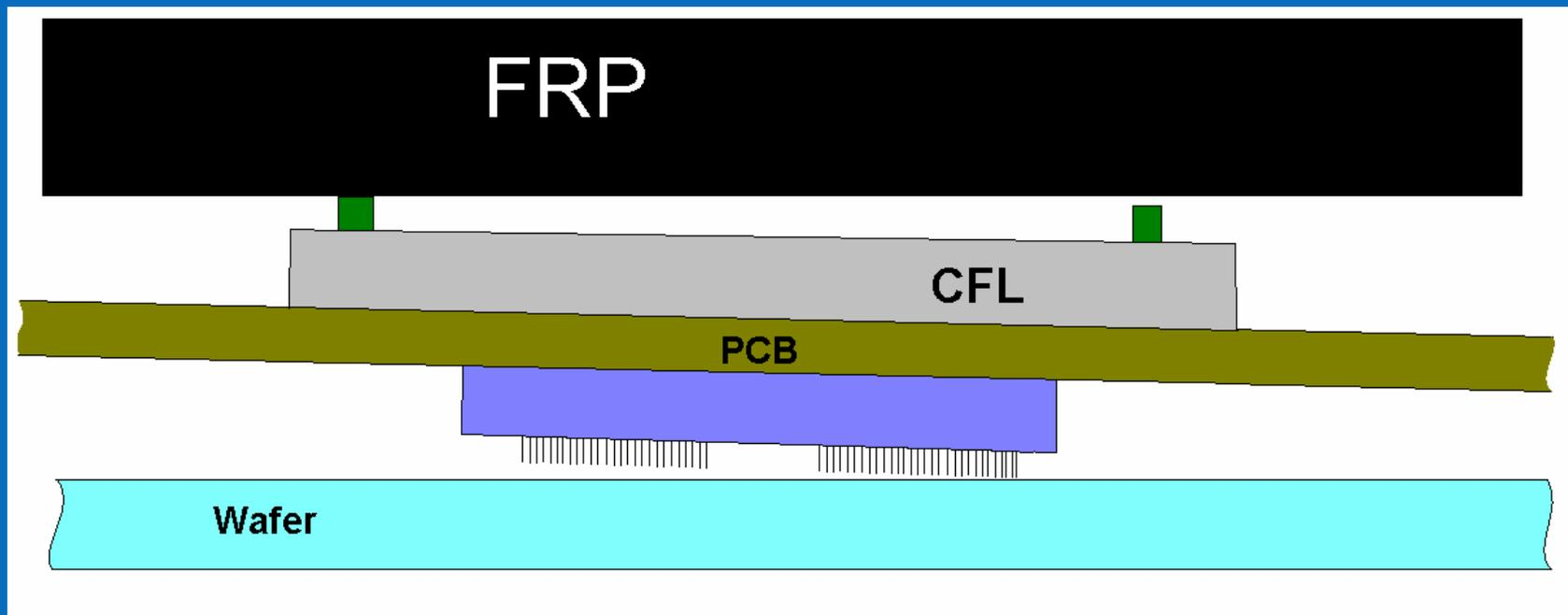
**Fig.2- Inconsistent CFL to FRP Contact**
