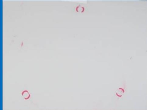
**b) Good Contact** → Red dots = good quality contact between FRP/CFL
