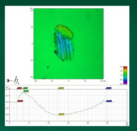
Scrub Profile @ 90C, 65um OD Pad damage ≤ 2% by volume, pileup not included
