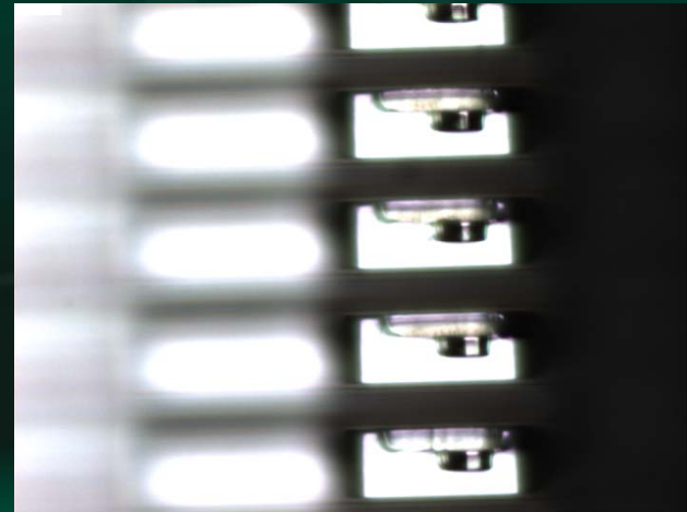
Picture showing Cantilever tip, placed by Laplace-3D process (80 \mu m pitch)
