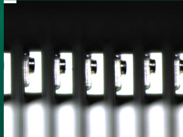
Picture showing Cantilever tip, placed by Laplace-3D process (80 \mu m pitch)
