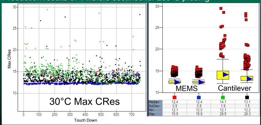
Device first released on dual site cantilever, then migrated to a x16 site MEMs probe card.
