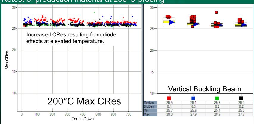
Results from high temperature testing show an increase of max CRes, but extremely stable with a StdDev of  $0.4\Omega$  or less.
