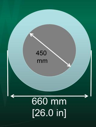
Connector area increased by 2.25x for additional signals
