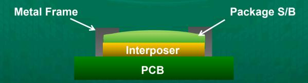
If stiffness of S/B is not sufficiently enhanced, the contact quality drops and there will be delay in conduction.
