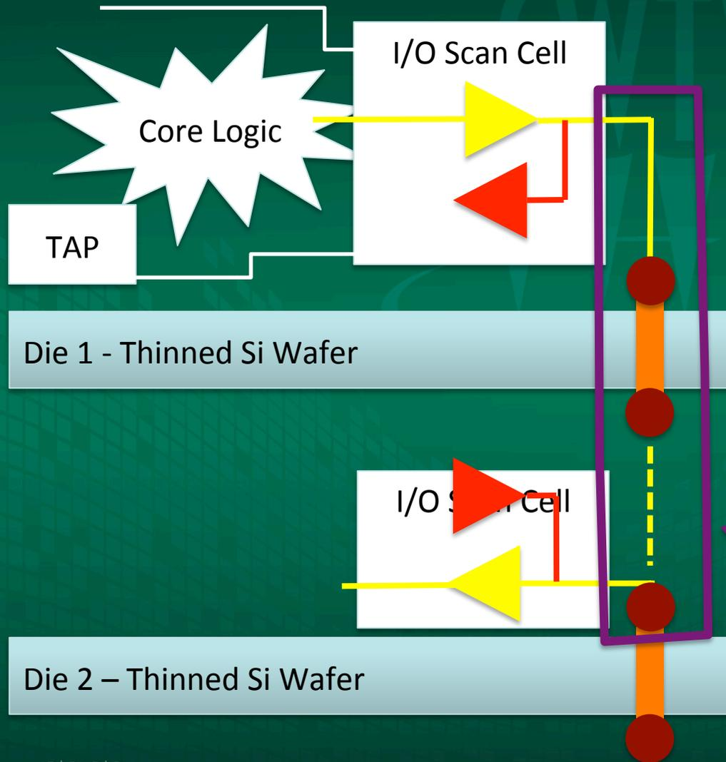
Add "feedback" structures to boundary scan cell to check drivers and receivers at wafer level to increase coverage.
