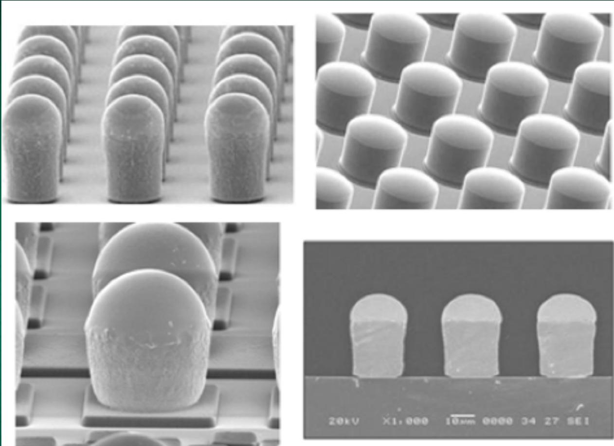
**Figure 1:** Examples of 40µm pitch copper pillar bumps capped with SnAg solder.
