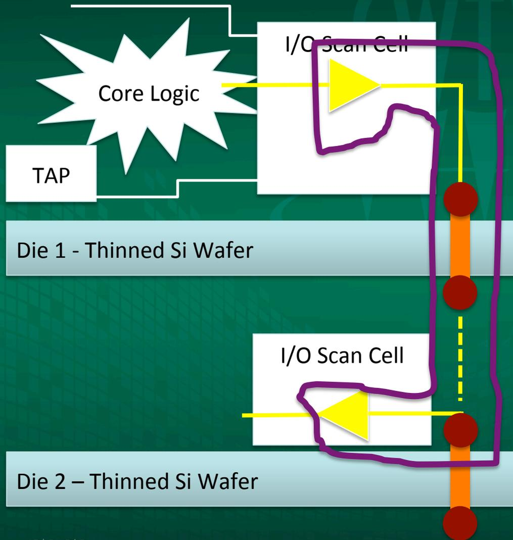
Inter-die connectivity (final driver, receiver, and interconnect) not tested during DFT wafer level probe.
