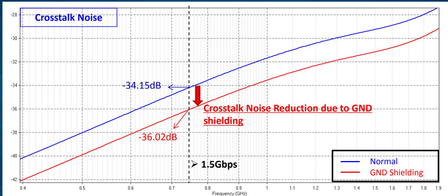
Reduction in Crosstalk Noise due to GND Shielding
