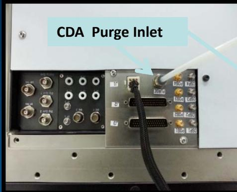
SC designed I/O panel with Tester Purge inlet & Backside Purge with Flow Meter and pressure gauge
