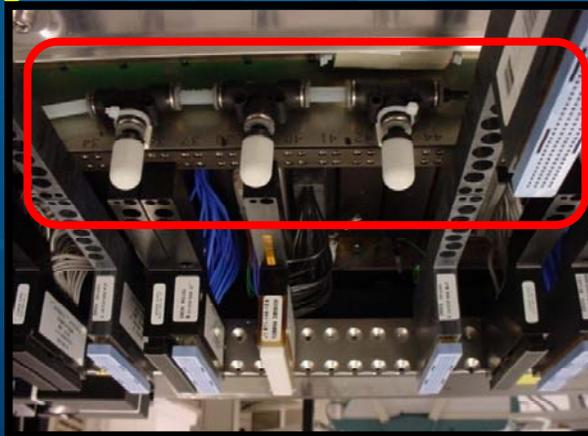
Back side purge diffusers attached inside IFLEX Test Head
