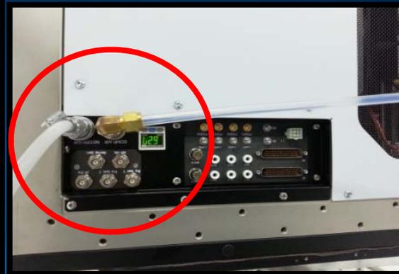
Backside Purge with Flow Meter and pressure gauge
