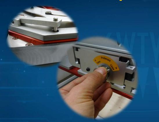
Probe card can only be captured or released after reaching secure destination
