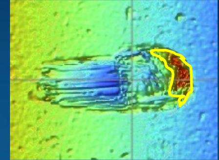
**Thin Pad Al:** Prow Area increases as both Tip Diameter and Force increase
