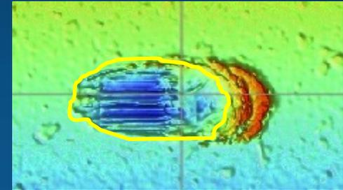
**Thin Pad Al:** Scrub Area increases as both Force and Tip Diameter increase
