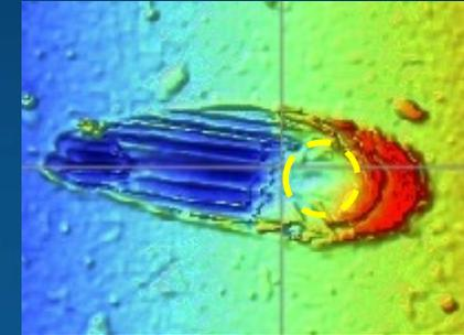
**Thin Pad Al:** Prow Diameter increases as both Tip Diameter and Force increase
