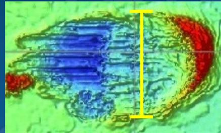
**Thin Pad Al:** Scrub Width increases as both Tip Diameter and Force increase
