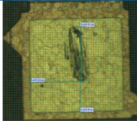
Probe marks sample produce using 4 mils Over travel
