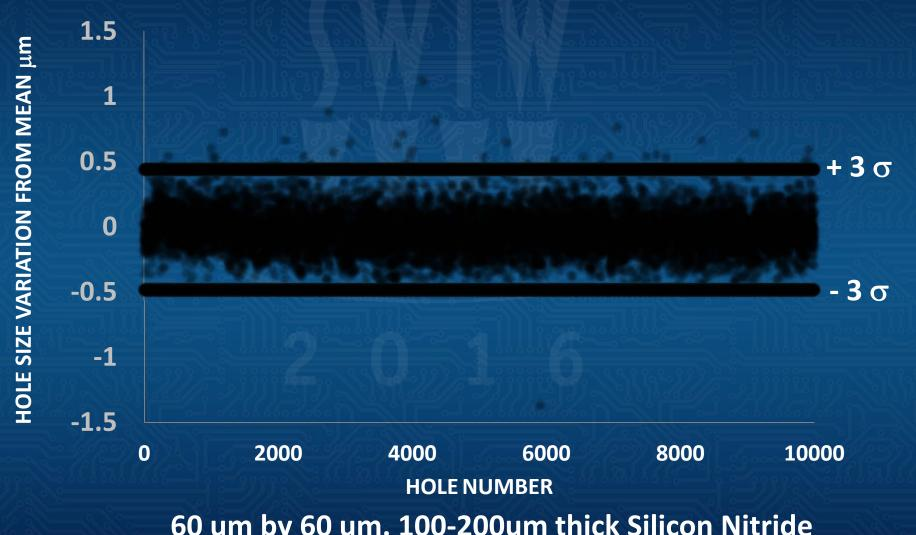
60 um by 60 um. 100-200um thick Silicon Nitride SW Test Workshop - June 5-8, 2016
