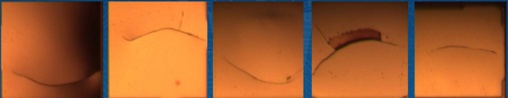
...these pads were actually cracked *due to severe ripple*
