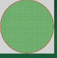
FULL WAFER CONTACT 16 touchdowns (-66,7%) 5014 DUT (+146%) ~ 300mm x 300mm active area Multi site efficiency of 98%
