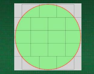
DUT OPTIMIZATION 18 touchdowns (-62,5%) 5808 DUT (+185%) 88 x 66 ( 79,2 x 59,4mm<sup>2</sup> ) Multi site efficiency 81%
