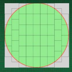
DUT OPTIMIZATION 48 touchdowns 2035 DUT 37 x 55 (33,3 x 49,5mm<sup>2</sup>) Multi site efficiency 87%
