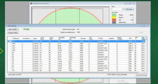
Best result = **5934 DUT** with **7 touchdowns** in SOLID layout = 69x86 ( 91,77 x 146,2mm<sup>2</sup> ) and highest multi site efficiency of 72%
