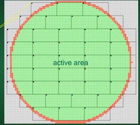
Multi site efficiency = % average of probe card touching active area dies overall on the wafer ( e.g. 84 % of 128 DUT )
