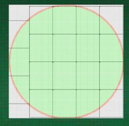
DUT OPTIMIZED 19 touchdowns 1978 DUT 43 x 46 ( 61,18 x 73,1mm<sup>2</sup> ) Multi site efficiency 80% DUT OPTIMIZED 7 touchdowns (-63,1%) 5934 DUT (+200%) 69 x 86 ( 91,77 x 146,2mm<sup>2</sup> ) Multi site efficiency 72%
