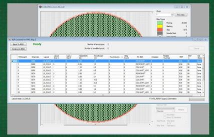
Best result = 6068 DUT with 5 touchdowns in a ~ 300mm x 300mm active area and multi site efficiency of 99%
