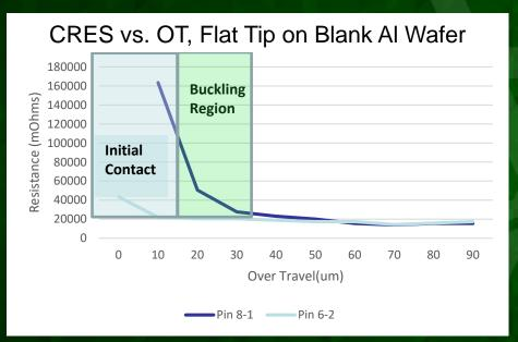
As a function of overtravel, resistance values stabilize as soon as the probe reaches its buckling point (2 probes shown reach same stable value)
