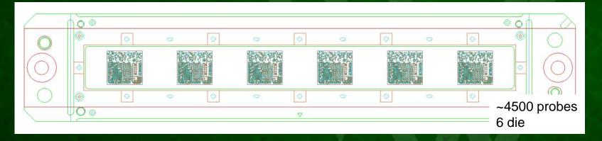
Vertical MEMS with frequency-capable guide plates can reach down to 106 um grid array pitch. And probe heads are able to support 8+ sites for complex, transceiver-type devices. Esher, Rhodes - SWTest | June 2-5, 2019
