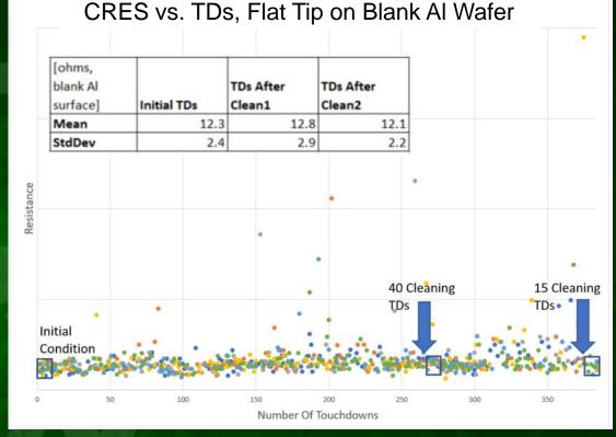
As a function of touchdowns, resistance values are relatively constant without any cleaning over many probing cycles, and can be returned to baseline values with an ordinary cleaning recipe
