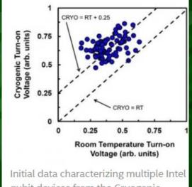
qubit devices from the Cryogenic Wafer Prober illustrate the increased voltage required for qubit gate "turnon" at cryogenic temperatures when compared with room temperatures across a 300mm wafer. (Credit: Intel Corporation)
