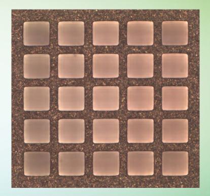
19 mil - 480 microns thick Silicon Nitride 18 mil – 460 microns thick Silicon Nitride
